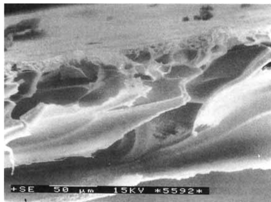
Figure 2 SEM micrograph of the cross-section of PAN- co -MA UF membrane type B.
